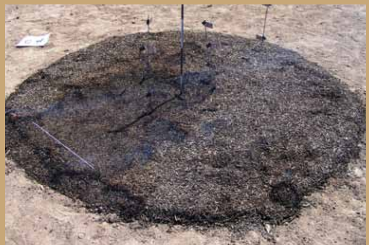
▶ Figure 6. The composted wood chip product, Fertile Mulch, primarily burned through smoldering combustion as indicated by the darker areas and smoke. It produced very little flame and had the slowest rate of fire spread of the mulch treatments evaluated.
